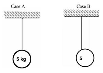
2. Determine tension in each cable. (Hint: There is more than one way to define the system.)
