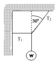
a. Write the equation for the sum of the forces in the x-direction. What is the value of  $T_2$ ?
